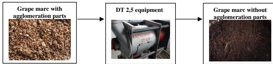
Fig. 2. Breaking grape marc agglomeration with DT 2,5 equipment
